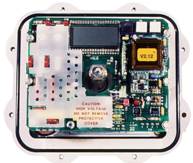
Three-button keypad for onsite calibration and functional setup.
